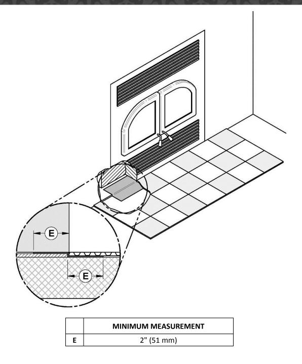
A noncombustible floor protection must be installed in front of the unit. For more details see **Section 1.3.2**: **Minimum Hearth Extension Requirements**.
